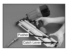
**Figure 3.** Sliding pusher toward the catch lever
